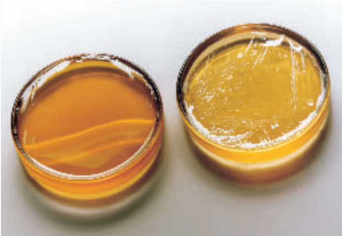
Surface structure of gels, produced with Classic Apple Pectin (left) and Classic Citrus Pectin (right)
